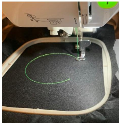
\*Place an oversized felt piece over the placement stitch. We recommend a color similar to the color you plan to use as the base layer for stitch step 3. You can tape the felt down outside the stitch area, but make sure the felt doesn't shift or bunch.
