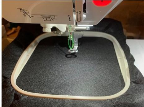
To begin: Hoop your cut away stabilizer. Tear away stabilizer is not recommended because the density of patches weakens this stabilizer. Multiple layers of tear away does not help.
