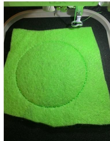
C. Stitch step 3 is the base layer and will take the greatest amount of time. Base layers are done in 2 passes, a bottom layer pass and then a more filled layer pass.
