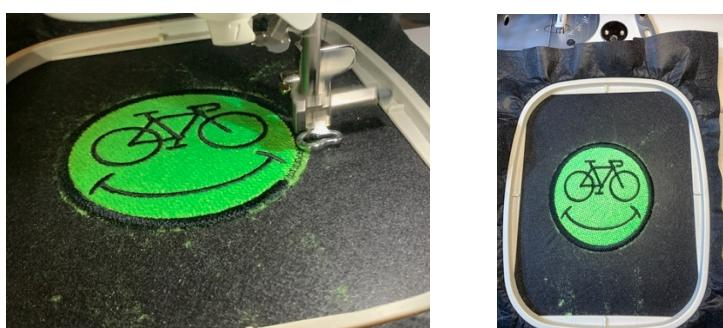
Once the final stitch step is done, you can remove the patch from the hoop. Trim the bulk of the stabilizer away.
